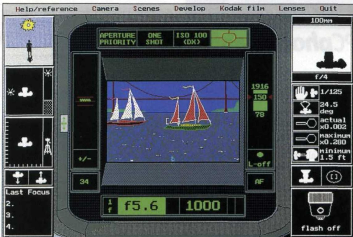
The screen shows the camera viewfinder and the scene you select, and allows you to select camera settings. Press the mouse button to take the picture. Across the top of the screen are the seven pull-down menus.
